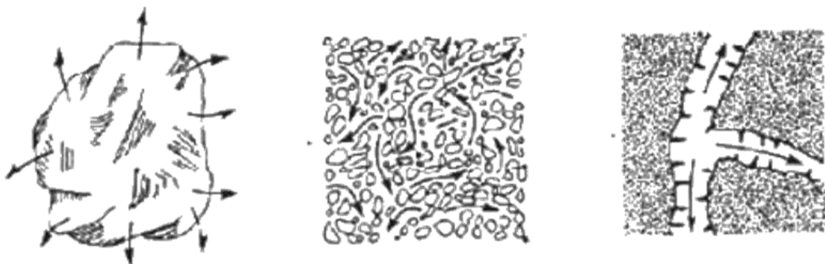
Fig. 1.B.5 – Transport mechanisms in coal seam methane: (a) Desorption from internal coal surface (b) Diffusion through the matrix and micropores and (c) Fluid flow in the natural fracture network. (From Reeves and Pekot, 2001)
