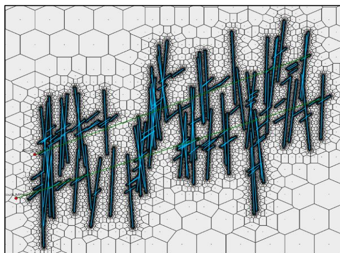
Fig. 1.H.11 – Stochastic distribution of DFN with two families crossed by two wells
